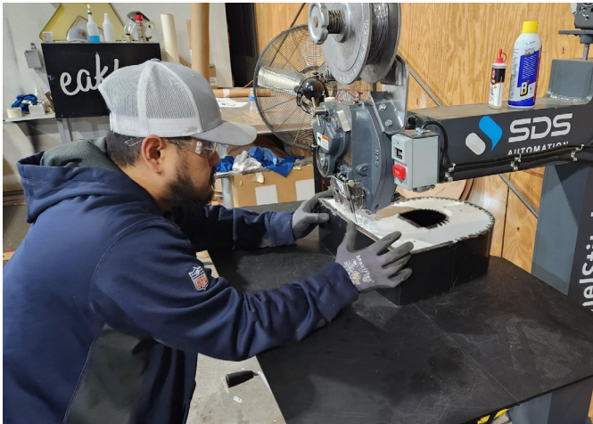
Porrith building channel letters.
